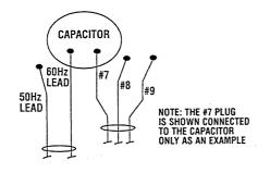
**CAUTION:** Make sure the insulating covers on the unused leads are in place and that the leads never come in contact with each other or come in contact with the case.
