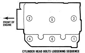
YLINDER HEAD BOLTS LOOSENING SEQUEN 2-Cylinder Engines
