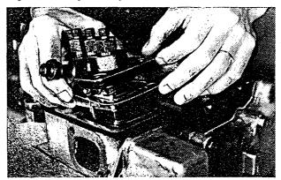
INSTALLING INJECTION PUMP 3-Cylinder shown
