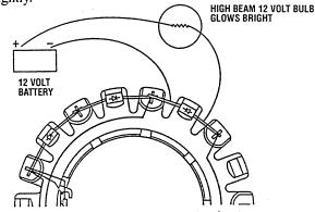
*Reverse the leads across the diode.* The diode should block voltage passing through it, and the headlight should not glow, or it may glow faintly.
