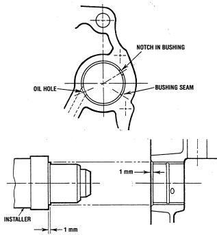
PRESS-FITTING CAMSHAFT BUSHING
