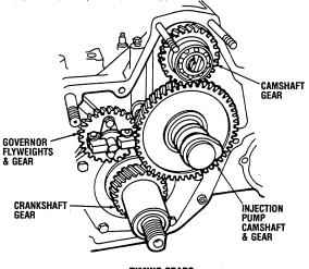
TIMING GEARS 2-Cylinder Engines
