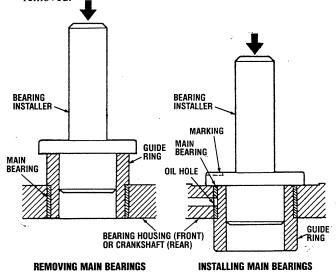
The main bearing must be pressed-in in such a way that the crankcase oil hole and bearing oil hole line up. The housing body has a marking on its collar. Set the bearing with the oil hole properly aligned with this marking, and then press in with the oil hole aligned with the crankcase oil hole. After setting, do not turn the tool and bearing. Be sure that the main bearing is pressed in with the outer area of the main bearing above the crankcase center.
