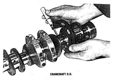
2. Check the crankshaft journals and pins for damage, seizure and other faults. If excessively worn or damaged, machine to the undersize diameter. At the same time, replace the corresponding main bearing or connecting rod bearing with the same undersize bearing. When machining a crankshaft journal or pin to the undersize one, be sure to finish its fillets to R2.5 mm. Check that all oil passages in the crankshaft are clean and open.
