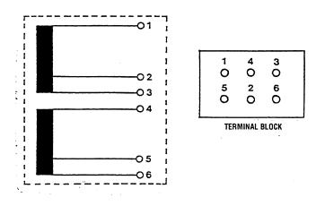
Residual voltage measured between line to neutral will be 4–6 volts AC between each pair of leads at the terminal block. This would be an indication that the stator windings are OK. Check exciter windings and artifically excite the generator.
