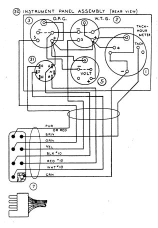
overheat condition exists and the operating temperature of the engine reaches 205°F, and sounds the alarm. The tachometer will register the engine speed as it takes impulses from the alternator as it charges. If the alternator does not produce a charge, the tachometer will not operate. The hourmeter will continue to record time. The hourmeter is on a separate 12 volt circuit.
