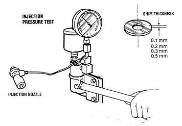
2. Chattering Test. For the chattering test, operate the tester lever slowly. If the nozzle sprays sharply and intermittently, the nozzle is considered good. The nozzle should spray fuel straight in its axial direction. A nozzle is defective if it sprays fuel in a wrong direction or in several separate strips. Also a spray in the form of particles indicates a defect. These defects may sometimes be caused by clogging with dust, therefore all parts should be carefully cleaned before assembly.
