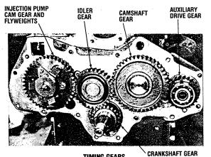
TIMING GEARS 3-Cylinder Engines Valve timing is as follows.
