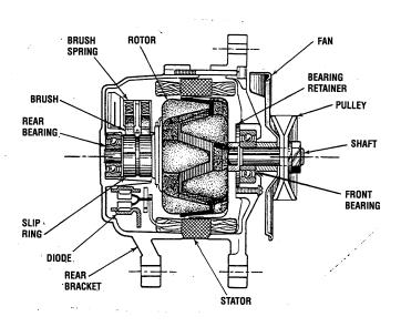
**NOTE:** The alternator connections and color coding described on the following illustrations may vary from earlier WEST-ERBEKE engines. Always refer to the wiring diagrams in this manual and also make a quick sketch of your alternator wiring before disconnecting for service.
