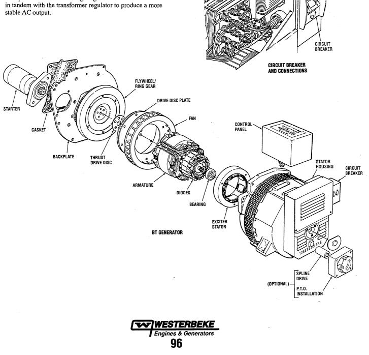
This troubleshooting guide will give you insights into problems which may be encountered with the WESTERBEKE 8.0 BTD brushless, transformer regulated generator. Most potential problems are covered in the text of this guide. Owing to the simplicity of the equipment and controls, this troubleshooting is relatively easy, once the relationship between cause and effect is understood.
