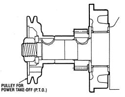
6. Temporarily install the sleeve stopper, washer (except for the P.T.O. pulley) and crankshaft pulley. Tighten the nut. Check the crankshaft end play. If the end play exceeds the specified value, recheck the thrust bearing. Also check that the crankshaft gear and sleeve are properly installed. After checking the end play, loosen the nut and remove the pulley and washer.
