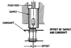
*The injection pump camshaft* is made of high carbon steel. Its cam surfaces are inductionhardened to improve wear resistance. The front end of the shaft supported on a ball bearing is connected to a gear. The rear end is provided with an Oldham's coupling groove for connecting to the oil pump drive shaft.
