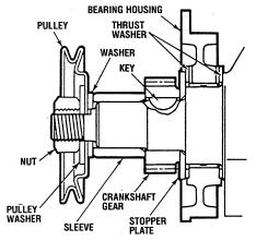
INSTALLING CRANKSHAFT GEAR & SLEEVE
