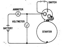
**CAUTION:** Use thick wires as much as possible and tighten every terminal securely. This is a solenoid shift-type starter which makes a rotating sound louder than that of a direct-drive type starter. When detecting starter rotation at the pinion tip, be careful not to come in contact with the pinion gear when it protrudes.
