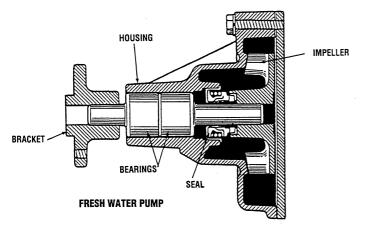
*The water pump* is a centrifugal impeller type and is mounted on the front upper part of the cylinder block. The pump shaft is supported on maintenance-free (grease-filled) double-row radial ball bearings.
