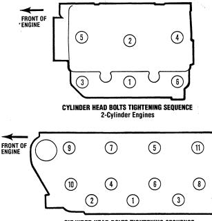
CYLINDER HEAD BOLTS TIGHTENING SEQUENCE 3-Cylinder Engines
