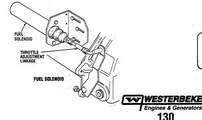
**A** CAUTION: Failure of the solenoid plunger to bottom in the solenoid will result in a failed solenoid.
