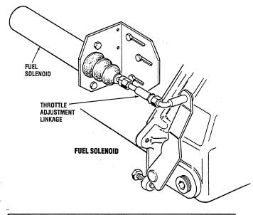
**A CAUTION:** Failure of the solenoid plunger to bottom in the solenoid will result in a failed solenoid.
