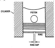
**MEASURING PISTON RING GAP CLEARANCE**
