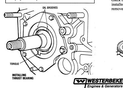
5. Install the outside thrust bearing in the bearing bore in the bearing housing, then install the stopper plate, crankshaft gear and sleeve. Install the stopper plate with the chamfered side facing toward the rear of the engine. Install the crankshaft gear with the stepped side facing toward the rear of the engine. Also install the sleeve with the chamfered square end toward the front of the engine.
