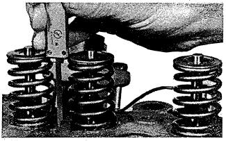
CHECKING FREE LENGTH OF VALVE SPRING
