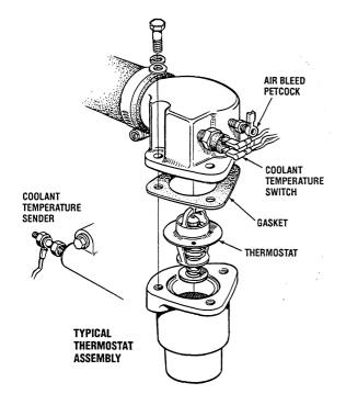
*Thermostat.* A thermostat housing is located on the cylinder head water outlet. Enclosed is a wax pellet-type thermostat. The valve opening temperature is not affected by variations of pressure in the cooling water passages.
