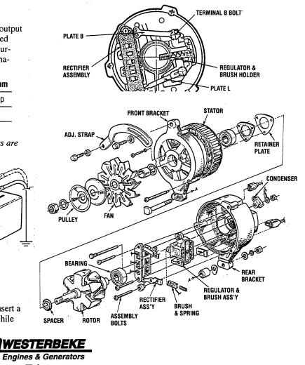
An alternate method for removing the stator winding, brush holder regulator unit and the I.C. diode rectifier assembly from the rear bracket. With the front bracket and rotor assembly separated from the rear half of the alternator:
