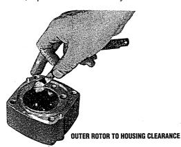
2. *Rotor clearance.* Check the clearance between the outer and inner rotors with a feeler gauge. If excessive, replace the rotor assembly.
