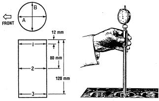
CHECKING CYLINDER WEAR
