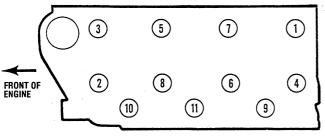
CYLINDER HEAD BOLTS LOOSENING SEQUENCE 3-Cylinder Engines
