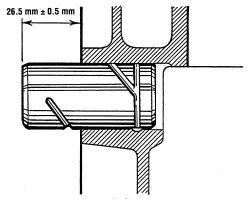
PRESS-FITTING IDLER GEAR SHAFT
