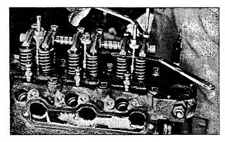
ADJUSTING VALVE CLEARANCE 3-Cylinder Engine shown
