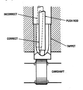
INSTALLING TAPPET AND PUSH ROD
