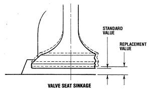
4. Check the valve seat inserts if provided, for proper fit. Replace any that fit loosely.
